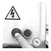
Press green key: the motor starts up and changes automatically from "star" to "delta" after about 3 seconds. The light of the green key is on.
