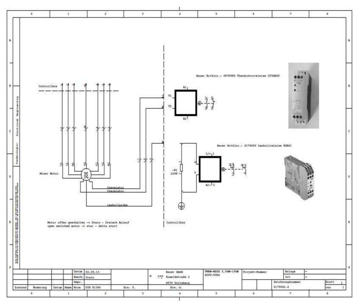
Wiring diagram 400 V 50 HZ star- delta start
