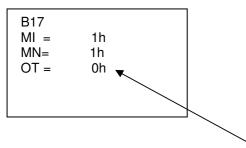
OT displays the consumed operating hours Do not change parameter MI and MN !! Press 2 times ESC for returning to the main menu
