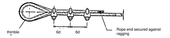
Number of wire rope clips needed for rope diameter of 8 mm: 3
